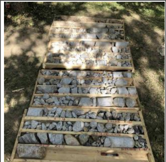
Photo 57: Drill cores at powerhouse
