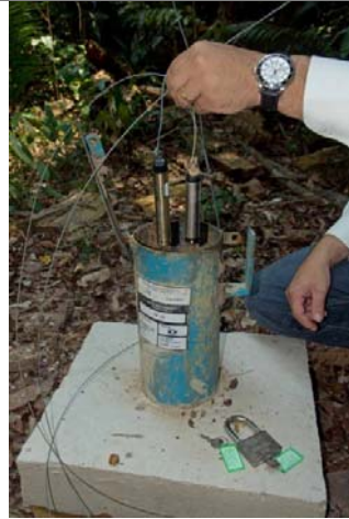
Photo 84: Ground-water measurement and sampling well.
