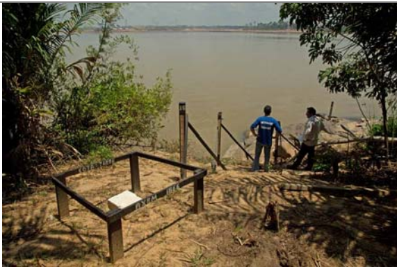
Photo 81: Runoff gauge downstream from the Jirau dam.
