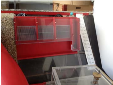
Photo 9: P-23 Intake structure on physical model of Gurgler intake
