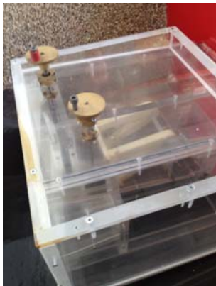
Photo 11: P-4 P-20 P23 Bottom outlet on physical model of Gurgler intake
