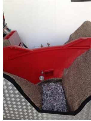
Photo 8: P-4 P-23 Physical model of Gurgler intake
