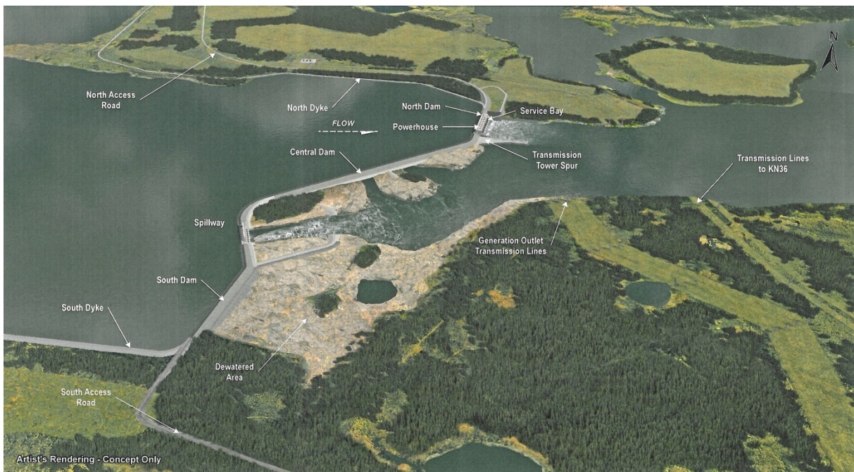
Figure 3. The same area as in the cover-page picture, but in an artist's rendering of the project layout, seen from the south. (from Keyask EIS).
