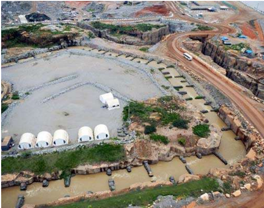
Figure 5. Aerial photo of fish-passage system
