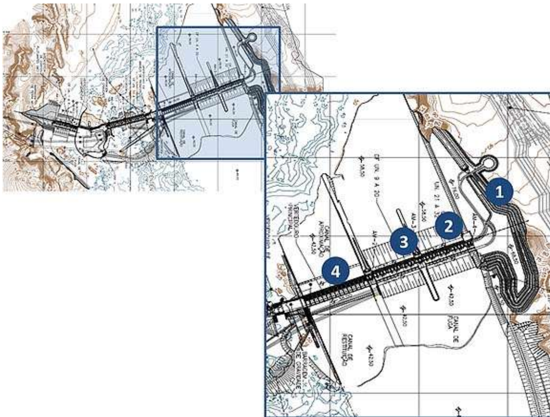
Figure 7. Left-bank structures of the Santo Antônio Project
