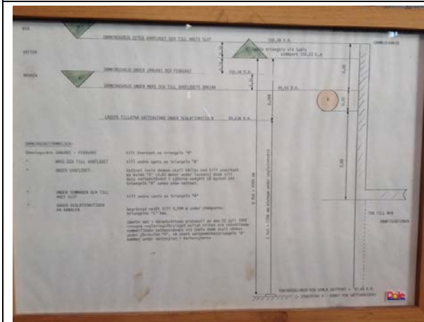
Photo 45: P-7, P-22 Graph of reservoir operating rules in Semla III powerhouse.JPG
